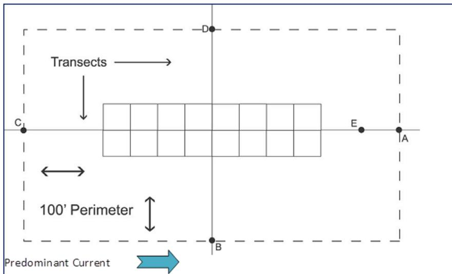
**Figure 6. Layout of allowable impact zone around net pens in Washington State and sampling stations for dissolved oxygen in this project.**
