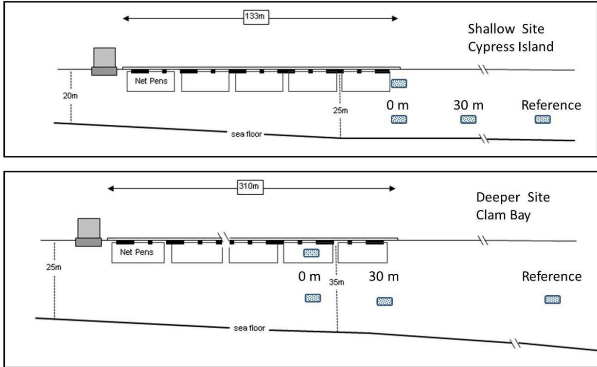
**Figure 3. Diagrams of the experimental layouts at each study site. Treatment and reference groups represented by blue rectangles. For Clam Bay, flow was tangential through the side of the cages and the 2D picture does not fully represent the arrays properly. See prior aerial image for spatial relationships.**
