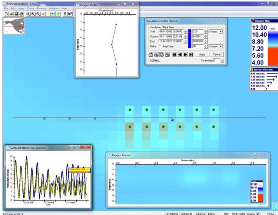
**Figure 9. Screen print of AquaModel simulation of oyster rafts current velocity of 1.5 cm/s (0.03 knots) shortly after the previous time period and with the vertical profile point placed through the lower left raft location.**
