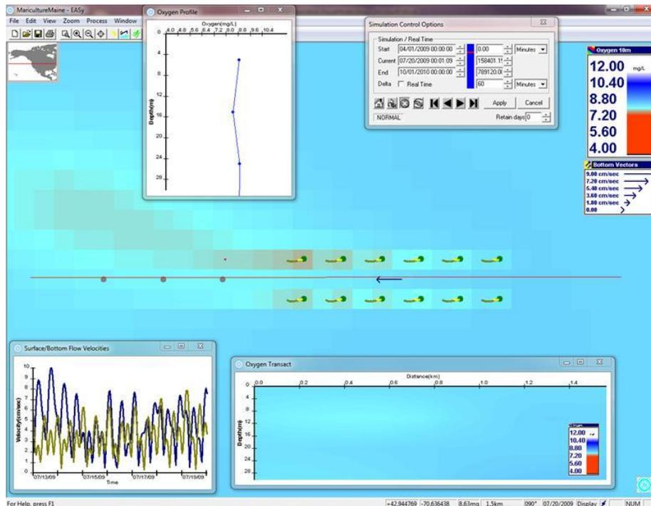
Figure 8. Screen print of AquaModel simulation of oyster rafts current velocity of 6 cm/s (0.12 knots) at the same time as above but with the vertical profile point moved 30m downstream.
